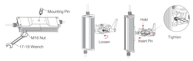
Option 2: Attach Power Adapter to the Yoke
